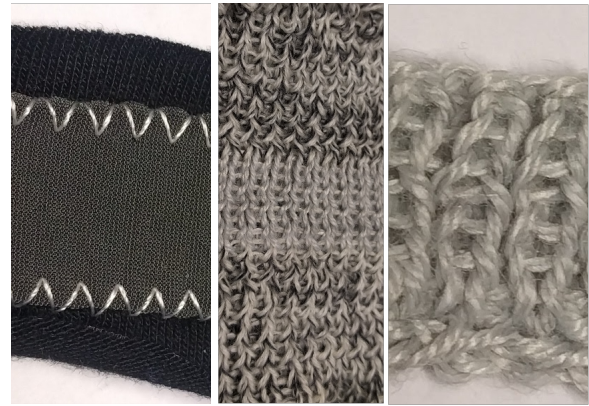
Figure 1: Photographs of each of the knit sensors. Not shown to relative scale. From left to right: Eeonyx fabric, machine knit, hand knit.
