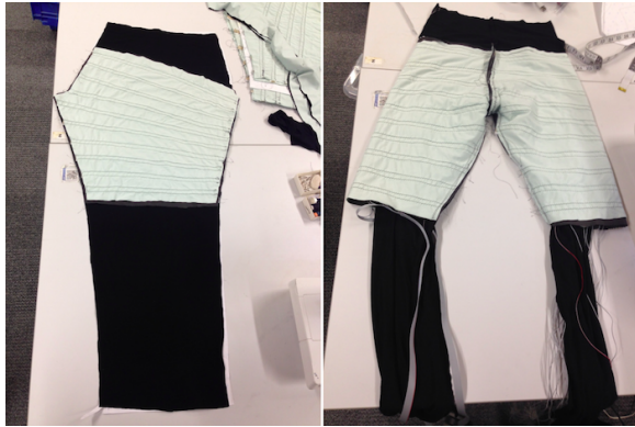
Figure 2: Left: pattern of one trouser leg, the back (buttocks) on the left with the more defined curve, and the front (crotch) with the steeper curve on the right. The sensor matrix ends around the knee (light blue fabric). Right: finished trousers turned inside out, before wires are inserted in tube panel on inside legs.
