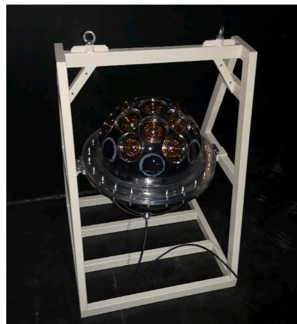
Fig. 5. Picture of the first preliminary mPMT prototype. The prototype is included in a white cage used to anchor the detector for sealing and operational tests performed at MEMPHYNO facility [35,36] at the APC Laboratory in Paris.
