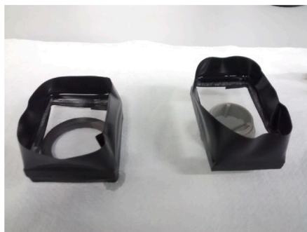
Fig. 4. Pictures of the acrylic samples with a 5 mm-thick optical-gel layer after its curing. Upon visual inspection, both samples appear transparent to visible light.
