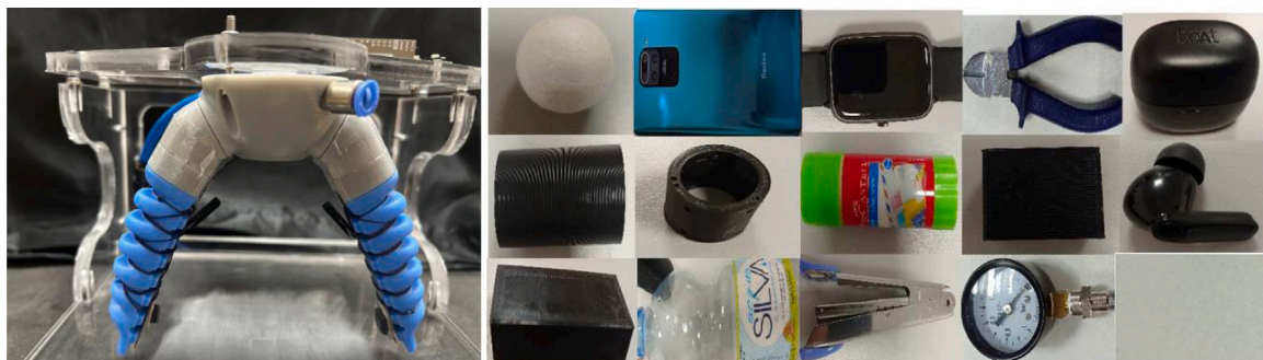
Fig. 8. Image of the gripper used and the objects. On the left panel are also visible the four sensor used.
