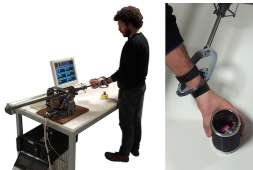
Fig. 1. Overall system employed for the generation of tremor composed by a haptic interface, controller and a novel end-effector spherical wrist.
