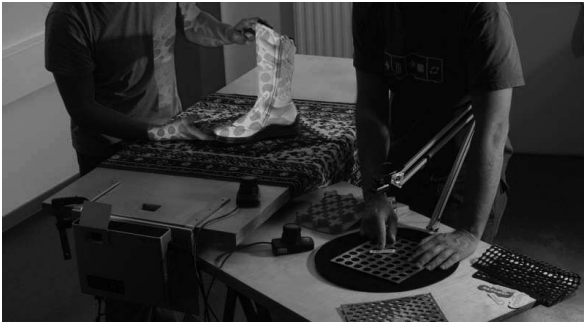
figure 1. The Skin setup consists of two interaction spaces. To the right and front you see the material palette whose function is acquiring and mixing visual materials. A webcam mounted on a swiveling arm grabs the materials. The object table on the left and back contains a projector that illuminates objects on the table with colored light.
