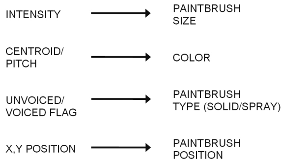
Figure 2: Mapping of voice features into graphic features.
