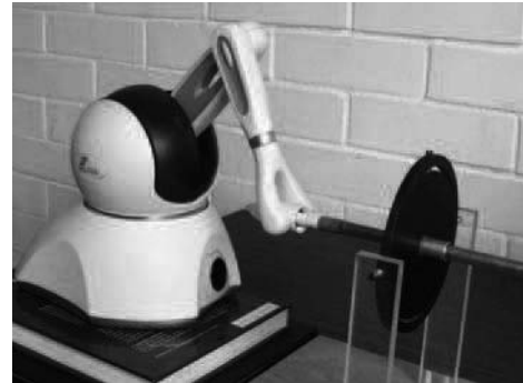
Figure 9: Scheme for adapting the resectoscope interface with an haptic robot for tactile feedback.
