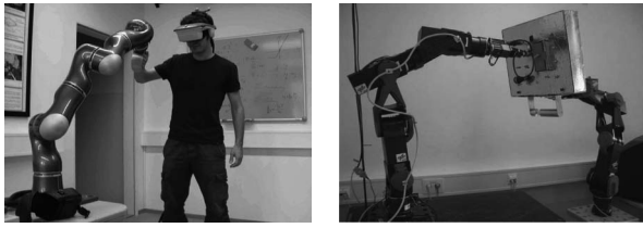
Figure 4: Telepresence test-bed. Operator moves DLR-LWR-III as the haptic display (left side). DLR-LWR-II (slave) performs operation on a movable satellite board (right side).
