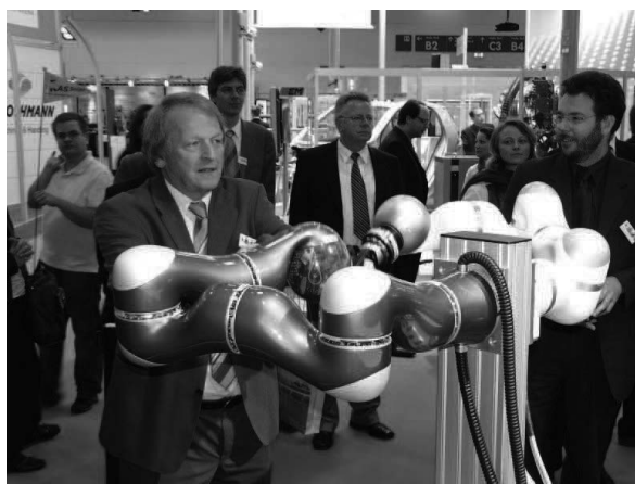
Figure 1: Two-robot system for bimanual haptic feedback.
