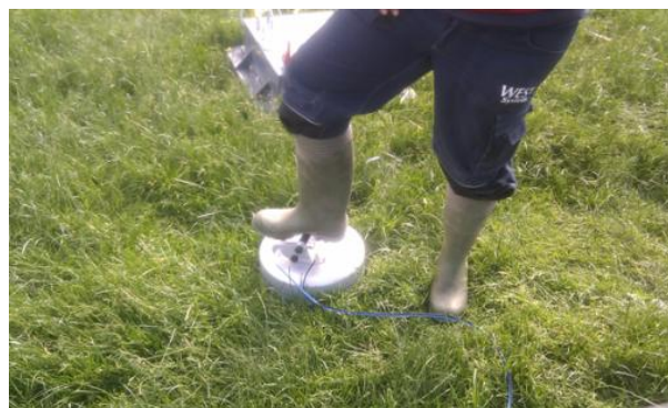
Fig. 14 Technique initially used to compress the chamber to the soil surface.
