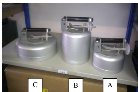
Fig. 3 Design of the IPNOA chambers.
