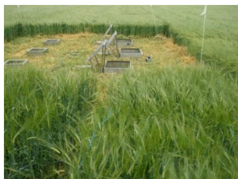
Fig. 7 Grignon devices with three manual chambers on left (area = 25 dm 2 ) and three automatic chambers on right (area = 49 dm 2 ). The height of chamber headspace was at mean 22.6 cm for the Auto chambers and 19.4 cm for the Manual chambers. INRA chambers differ on IPNOA chamber by their volumes and areas more wide. Their frames are inserted to a deep of about 7 cm into the soil.
