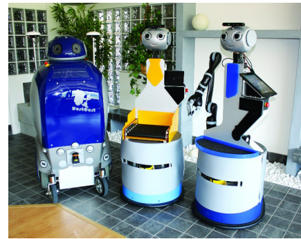
Figure 4: The three platforms used in the experimentation: the outdoor robot Oro (left), the condominium robot Coro (center) and the domestic robot Doro (right),
