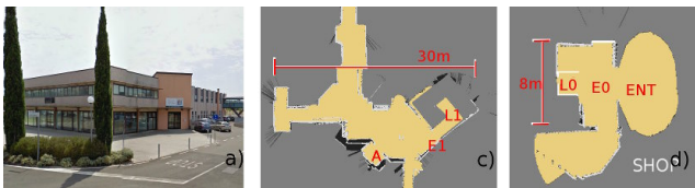
Figure 6: DomoCasa Living Lab of the Biorobotics Institute (Scuola Superiore Sant'Anna, Italy). The Biorobotics Institute (left); ROS map of the first floor (middle); ROS map of the ground floor (right). Both maps shot the symbolic locations used in the plan.
