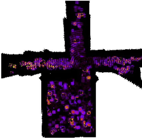
Fig. 4. Affordance Composite Map of 70 maps. Clearer values show higher probabilities of having humans in those locations.
