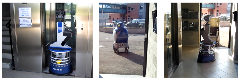
Fig. 5. Left: coro - a SCITOS-G5 from Metralabs; Center: doro - a DustBot from Robotech Srl; Right: The robots exchanging goods.
