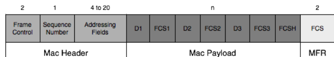
Fig. 2: Standard IEEE802.15.4 data frame with data payload fields required by the proposed FEC scheme.
