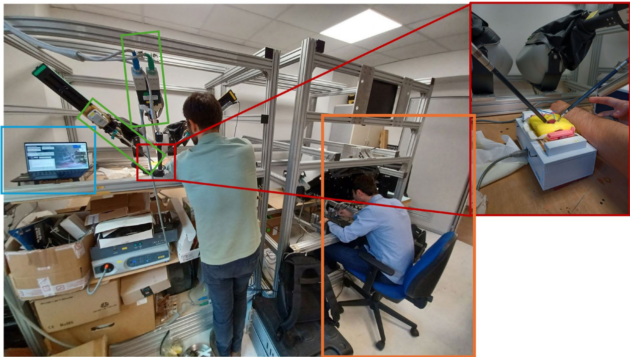
Fig. 1 Dry-lab training setup in Pontedera using the dVRK platform and sensorized vascular simulator. The green boxes highlight the robotic arms, the blue box shows the computer-based sensor monitoring system, the red box shows the simulator, and the orange box highlights the surgeon in training.
