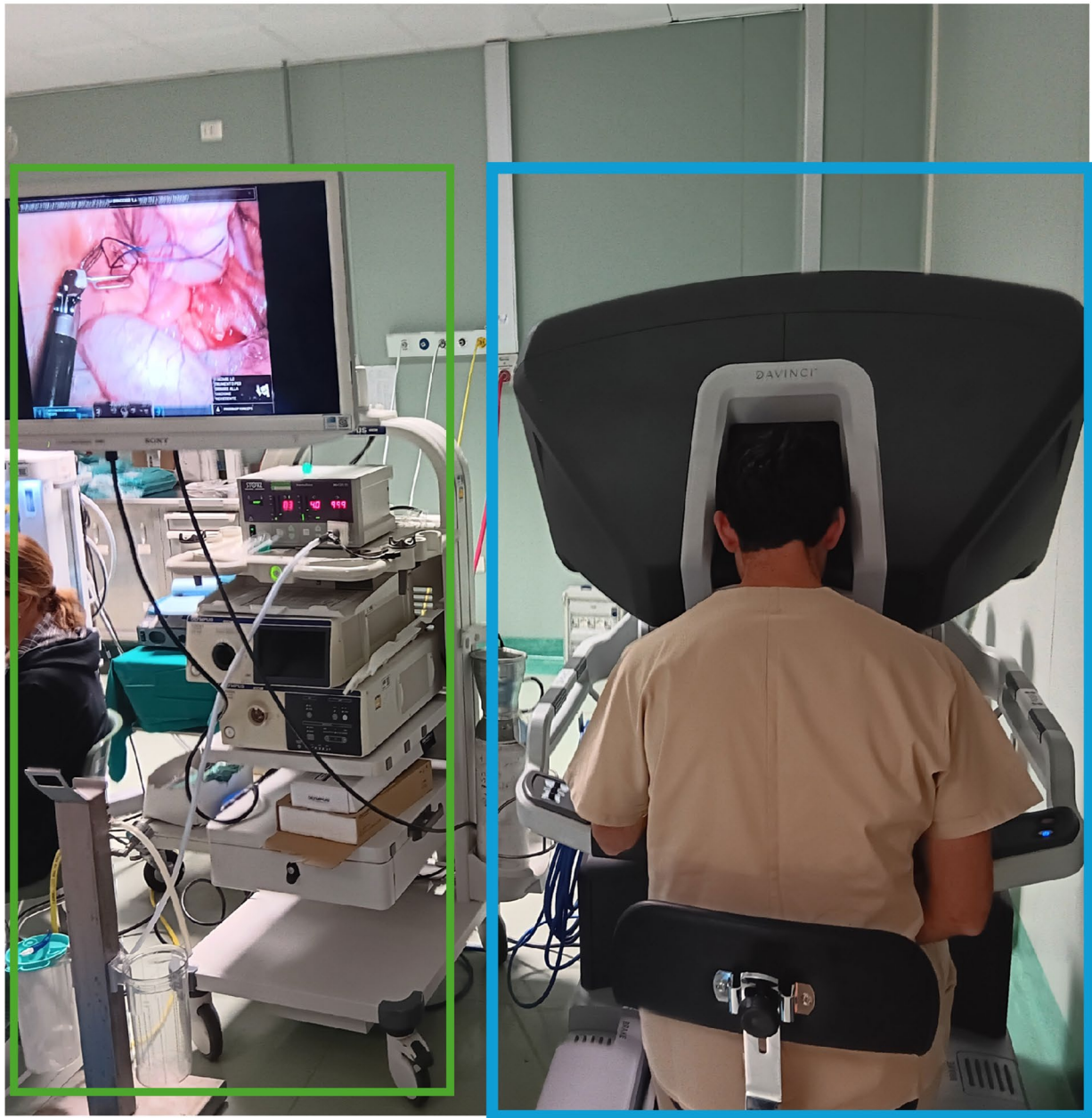
Fig. 2 Animal-lab validation in Grosseto using the da Vinci Xi platform on a porcine model. The blu box highlights the surgeon operating at the robotic console.
