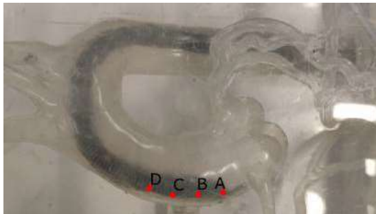
Fig. 2 The positions of the 3Flex inside a realistic aortic phantom for performing the catheterization using an MC.
