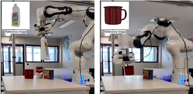
Fig. 5. Grasping of different objects of the YCB-V [2] dataset, from the provided reference image (top-left in each picture), using the presented InstantPose method.
